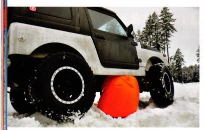
Let the exhaust do all the work with an exhaust jack.
